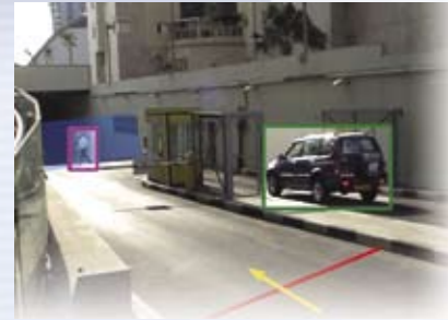
Nextiva automatically identifies and classifies objects within a scene, like the man and the car in this video still.
